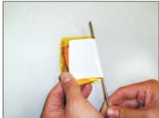
Picture: .IPC-TM-650 2.4.5.1 Flexibility; solder mask
